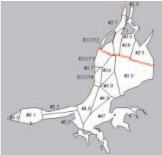
FIGURE 93. ZONES OF INFLUENCE CALCULATED WITH THE THIESSEN POLYGONS METHOD.
